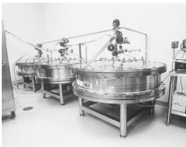
Fig. 5. Industrial fractionation by gel filtration using three BPSS columns (30x140 cm i.d.) in series giving a total bed volume of 1500 liters. By courtesy of R. Hershberg.
