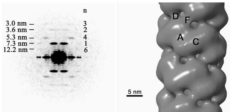
**Fig. 3** **a** The average power spectrum of the 853 selected aligned images. Five layer lines corresponding to the spacings shown on the left are visible. These are interpreted as being of the Bessel order shown on the right. **b** The three-dimensional reconstruction of the density from the images using the iterative helical real space method. The locations marked *A*, *C*, *D*, and *F* are the interfaces between subunits. Lines between points of type *A* and *D* and between points of
